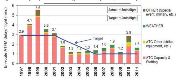
Figure 2-2: Origins of en-route<sup>21</sup> Air Traffic Flow Management (ATFM) delays<sup>20</sup>
