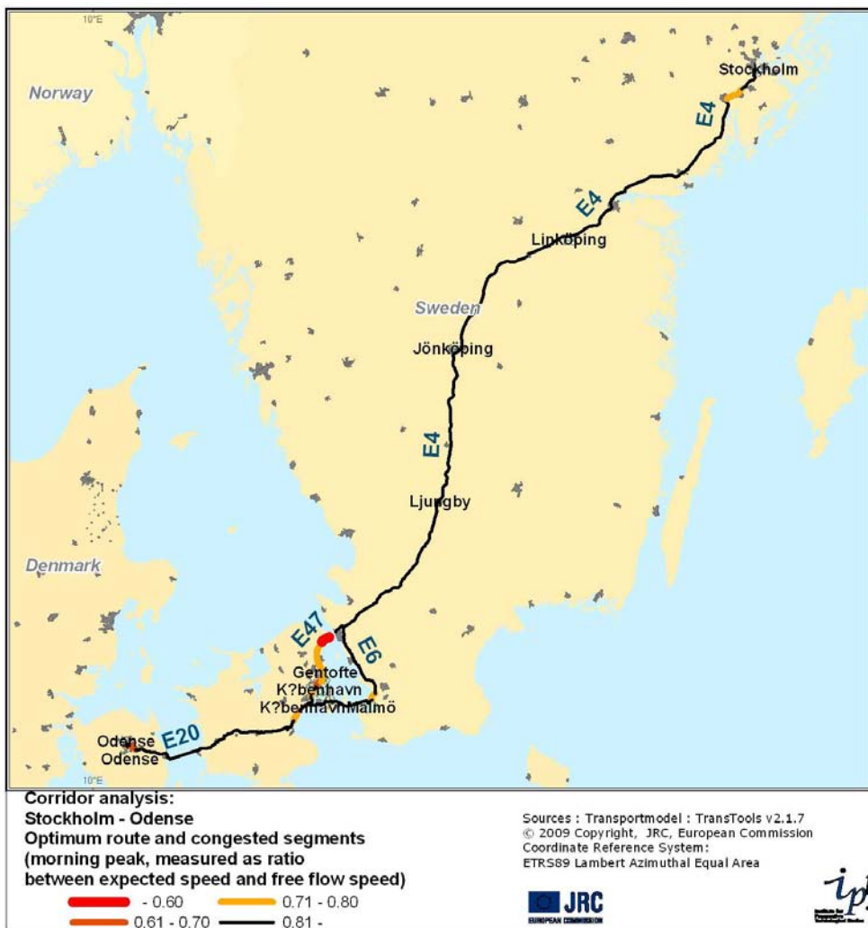
Figure 14: Optimal route for Stockholm - Odense corridor and congestion levels
