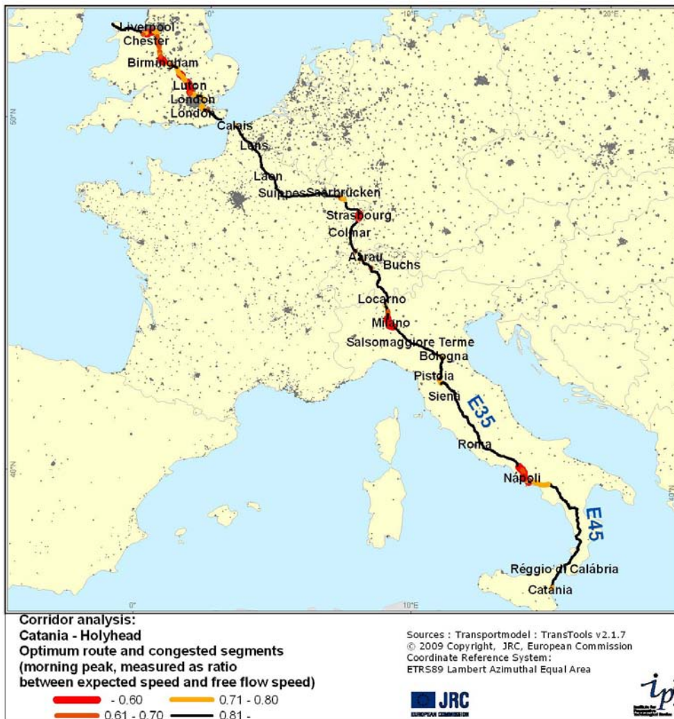
Figure 8: Optimal route for Catania - Holyhead corridor and congestion levels
