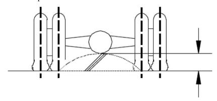
4.2.2. Where appropriate, the measurement of ground clearance shall be conducted on each of the several axles of a group of axles.
