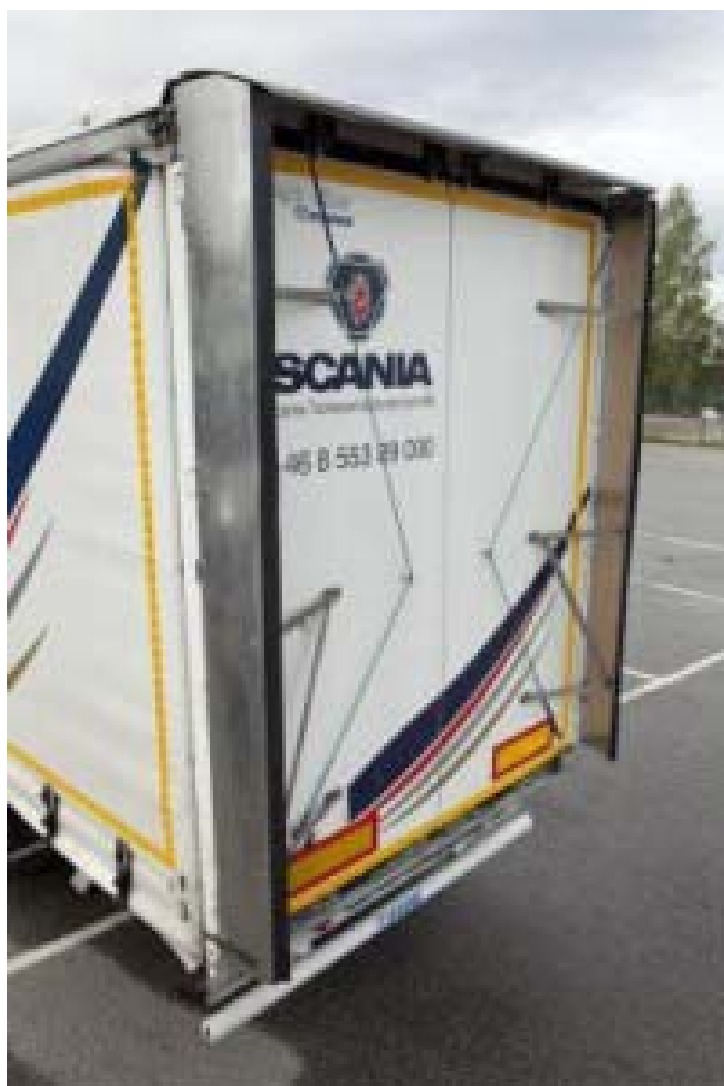
Figure 3: 500 mm deflector under test
